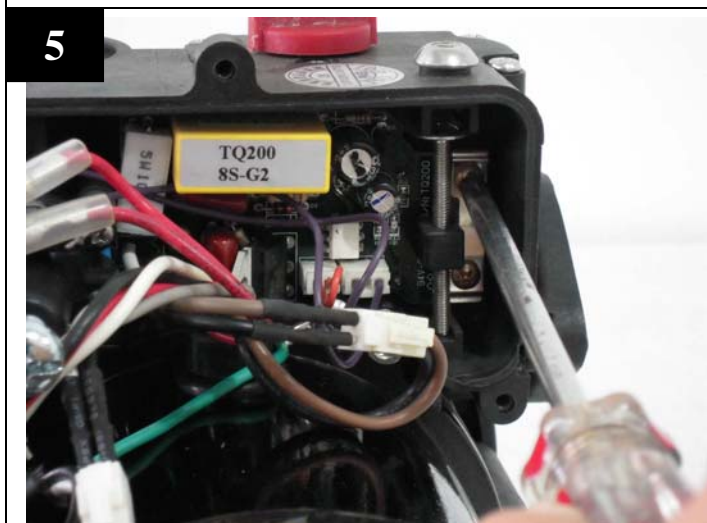
Loose the screws that hold the control board.
