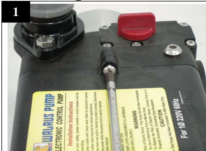
Loose the screws and remove the terminal box-set.
