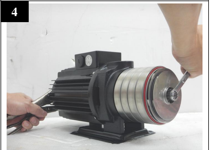
Using wrench to loose the lock nut.
