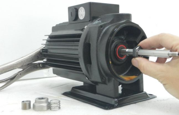
Remove the rotary parts of mechanical seal.
