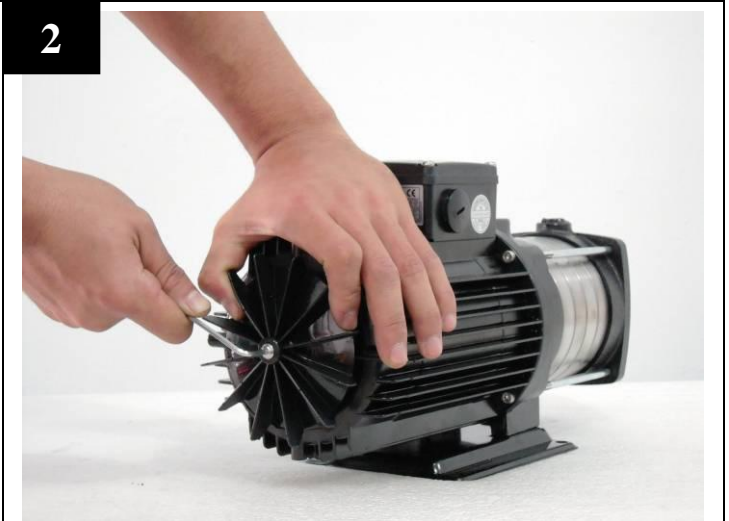
Using Allen wrench to remove the motor fan.
